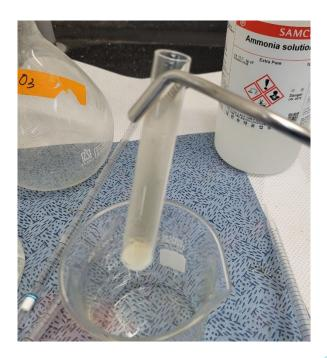
**3. Confirmatory test.** Slowly add drops of conc NH<sub>3</sub> (Caution: Avoid inhalation or skin contact!) to the solution from Part D.2. The deep-blue confirms the presence of  $Cu^{2+}$  in the solution.
