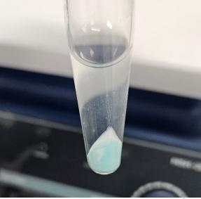
**2. Confirmatory test.** Wet the precipitate to a moist paste with a drop of 6 M HCl and perform a flame test. A fleeting yellow-red flame is characteristic of calcium ion and confirms its presence.
