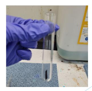
**2. Oxidation of copper metal.** Transfer the test tube containing the copper metal to a fume hood. Add drops of 6 M HNO<sub>3</sub> (**Caution:** 6 M HNO<sub>3</sub>, *cause sever skin burns, and the evolved NO gas is toxic*) until the copper metal completely reacts. Be patient; some heating in a water bath may be necessary.
